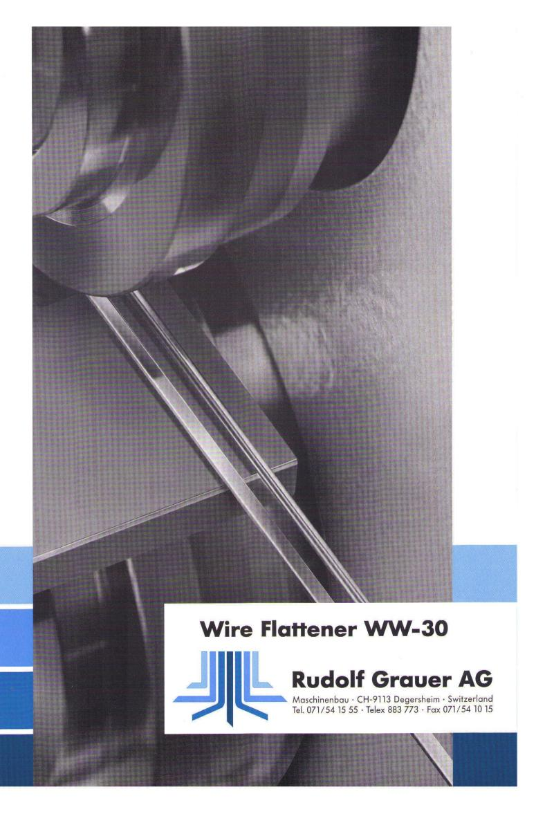
**The Wire Flattener WW-30** serves for flattening of round wire. With the two independent and separately driven flatteners two wires, also with different speeds, wire diameters or flattening depths can be produced simultaneously.
